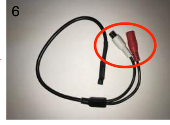
6 Find the Microphone White RCA (Female) and Red Plug (Female)
