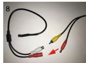
8 Plug Red Plug (Male) from Microphone Extension into Red Plug (Female) on Microphone
