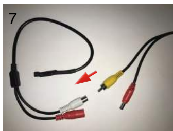
7 Plug Yellow RCA (Male) from Microphone Extension into White RCA (Female) on Microphone
