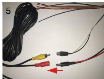
5 Plug the Black Plug (Male) from the Power Harness into the Red Plug (Female) on the Microphone Extension
