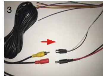
3 Plug in the Yellow RCA (Male) from Microphone
